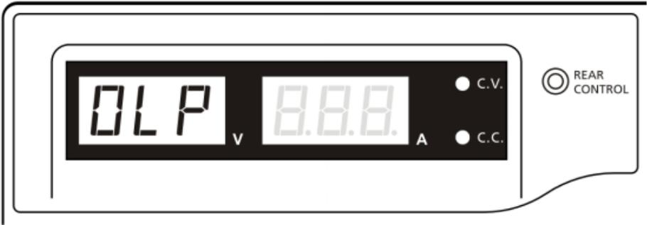
**Figure 15 - Overload Protection**
