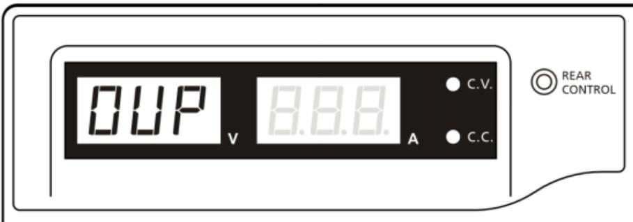
Figure 13 - Overvoltage Protection
