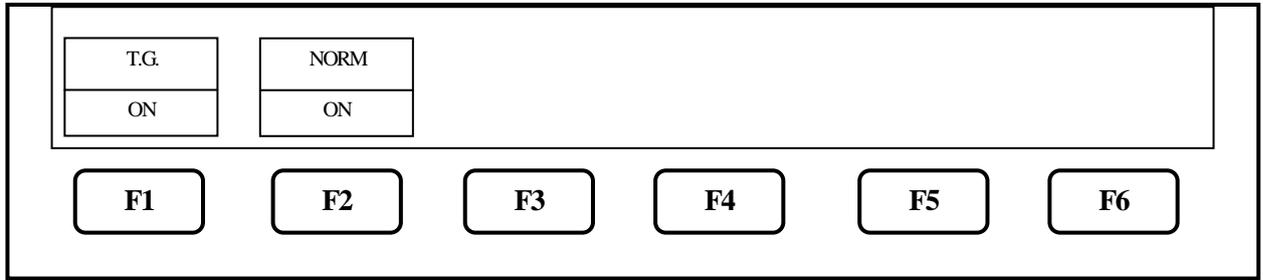
2. Each time F1 is pressed, T.G. output is alternately switched to ON or OFF.
