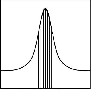
This is based on the sum of power in the specified bandwidth. The center frequency of the reference carrier is set by [F4].
