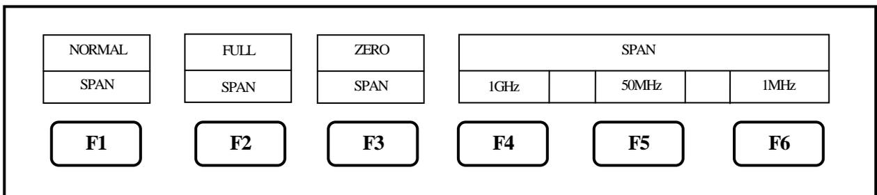
By operating **SPAN** →
