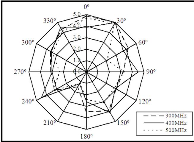
Antenna gain vs. Frequency
