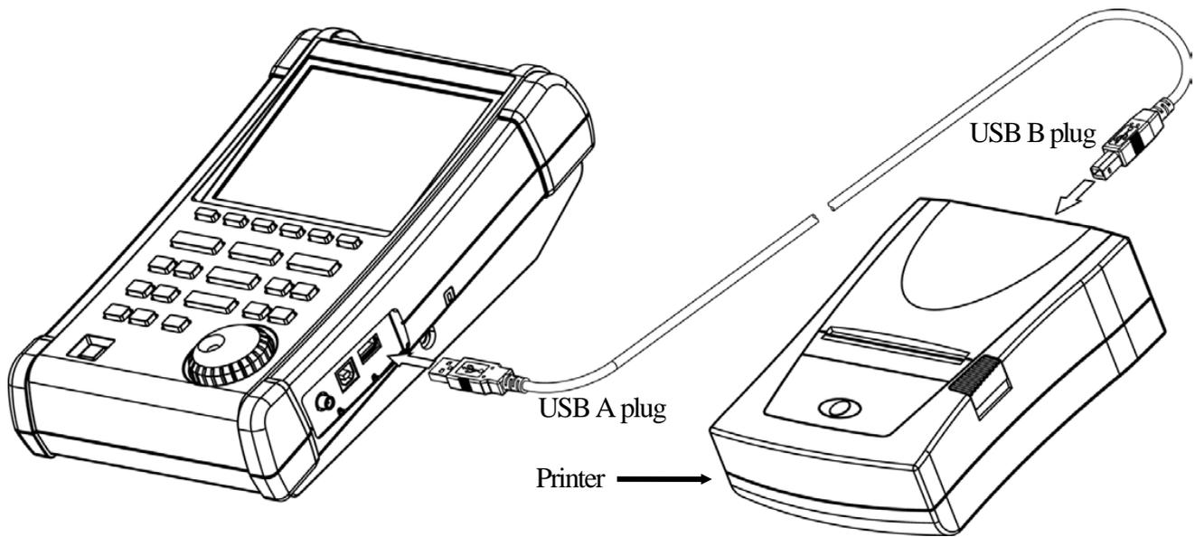
\* Turn on the power of the 2650A/2651 series unit first. After that, turn on the power of USB printer. Otherwise, it will not work correctly.
