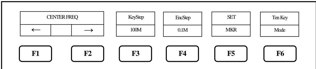
\* Center frequency setting range: 0 to 3.3 GHz for 2650A/2652A/2651, 0 to 8.5 GHz for 2658A
