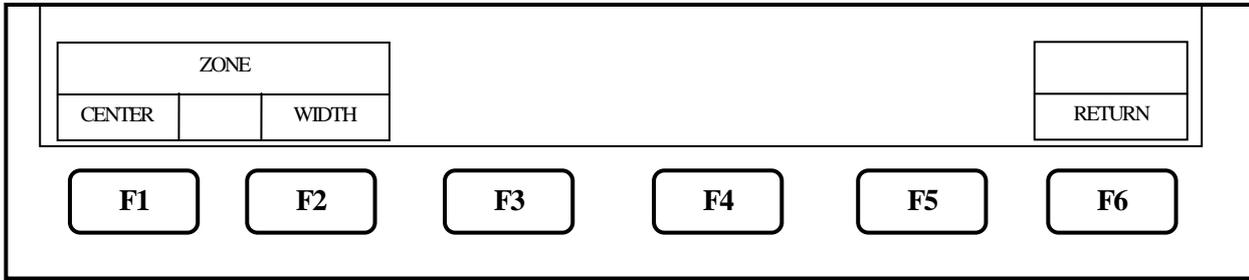
At the Zone mode, the marker automatically moves to the maximum peak point within the range set beforehand. When entering this mode, the zone is displayed with thin blue shadow in the spectrum display area.
