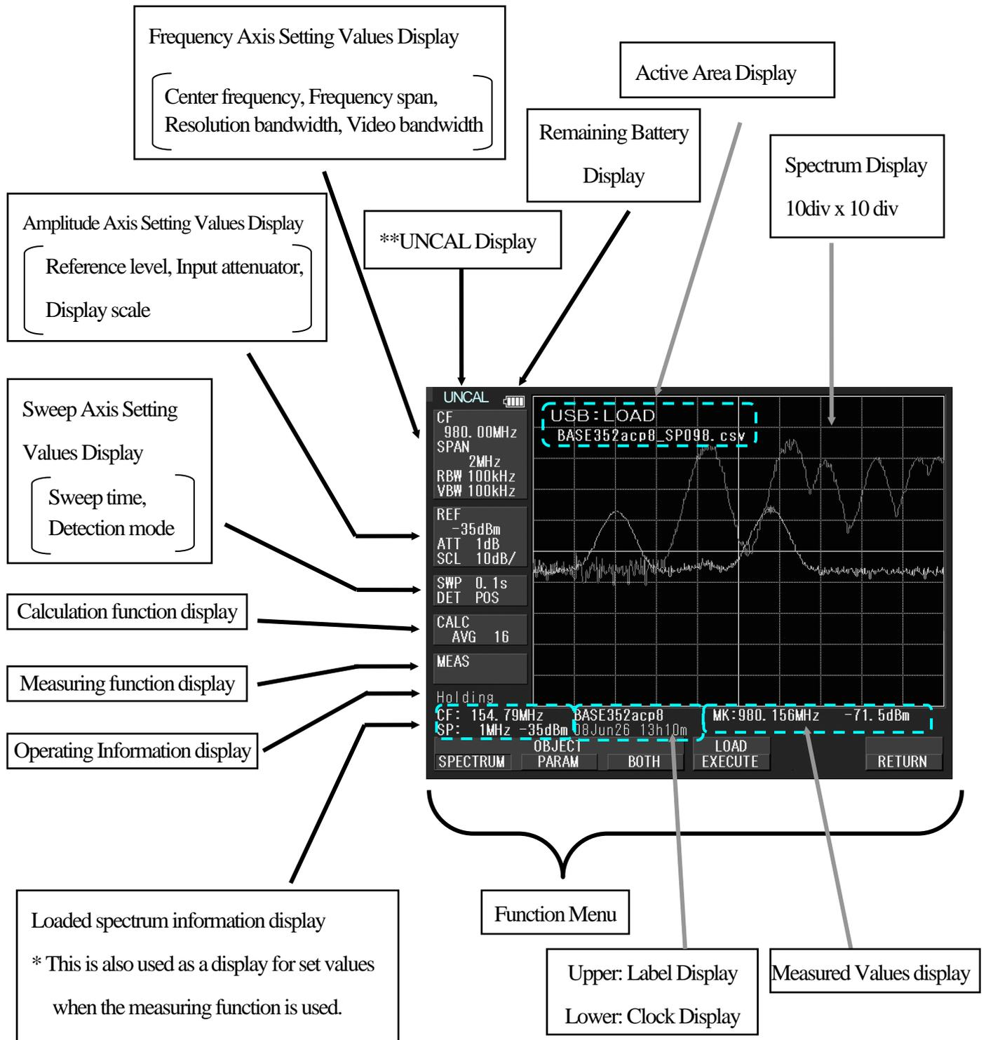
\*\*UNCAL is displayed when a normal measurement cannot be done due to sweep rate being too fast. In such cases, slowing down the sweep rate will change this indicator.
