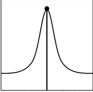
This is based on the power of peak on the screen. The center frequency of the reference carrier is automatically set to the peak on the screen.
