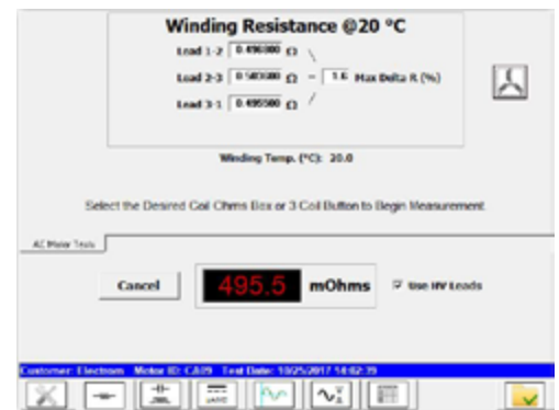
\mu\Omega measurement of 3-phase motor
