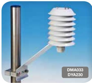
The meteorological sensor DMA033, closed in its anti-radiation screen DY230, can be connected to MSB and STB modules. The sensor's accuracy is 1/3 DIN (0,1°C) and is equipped with L.10 m cable.
