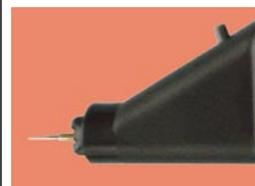
The MINI E-field generator cannot be used for compliance testing. Measurements on standard test stations are necessary to determine standard disturbance immunity values. Practical experience, however, allows assessments.
