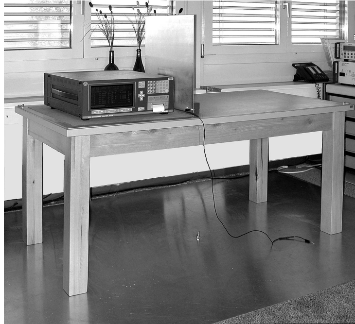
Fig. 1 ESD test set-up as described in IEC/EN 61000-4-2. Note Ground Reference Plane (GRP) connected to earth (ground)
