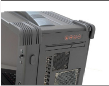
View of the Corner Shock Isolation Bumpers
