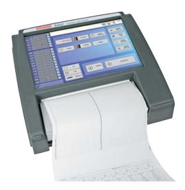
To suit your specific and various applications, you can configure and select all printing parameters (including plotting mode f(t) or text), paper speed (1mm/h to 100mm/s), number of traces or grid pattern.
