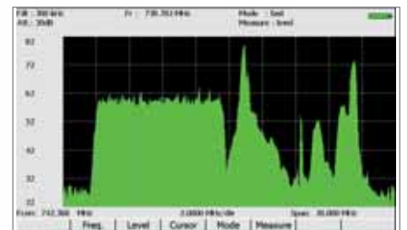
Spectrum analysis in "expert" mode for adjacent channels investigations.
