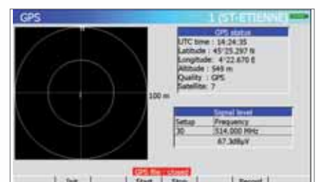
GPS function For 7866HD-T2, to map your measurements.
