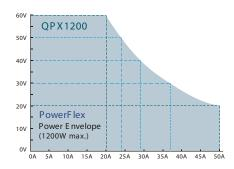
The QPX1200S & SP offer users a level of flexibility that cannot be achieved with conventional laboratory power supplies. They can therefore perform the task of many different power supplies.
