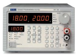
Local operation convenience features of the TSX-P series include a auxiliary display for displaying other data such as increment values, OVP level, or watts
