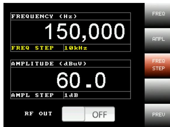
Fig.16: FREQUENCY STEP adjustment
