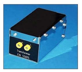
The output impedance of the transformer, when the input is terminated by  $50\Omega$ , is  $150\Omega \pm 10\%$ , with angle phase less than 10°. The insulation of the transformer is checked as CISPR 15 requirement, in the f=150kHz÷1605kHz frequency range. The transfer characteristic is flat,  $\pm 0.5$ dB.
