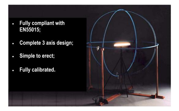
**TLA-300** is a calibrated **2-metre large loop antenna** manufactured to comply with product standard **CISPR 15** and **CISPR 16-1**. The calibrated frequency range of the TLA-300 is 9kHz to 30MHz and each antenna is supplied complete with antenna factor data so that it can be used with any EMC receiver or spectrum analyser capable of antenna factor compensation. The performance of the loops is matched to the 'ideal' loop curves as shown in EN 55015 using the prescribed test set-up.
