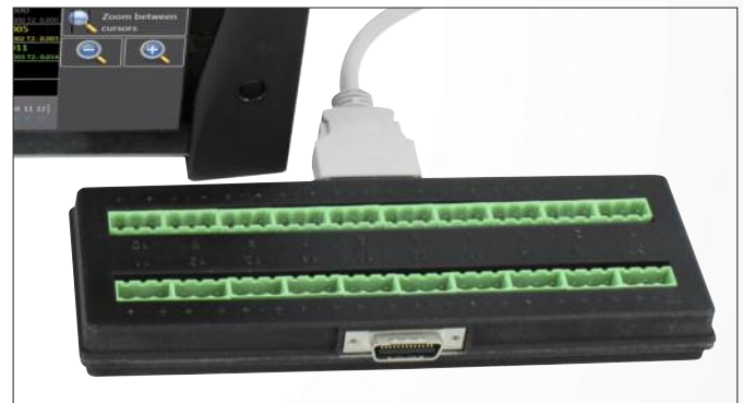
20 analogue channels board P/N: 902401000
