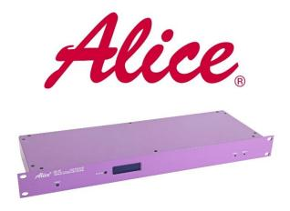
The Alice LTC timecode distribution amplifier is a 19" rack mounted unit that provides six balanced outputs via Neutrik XLR connectors and six unbalanced outputs via 75ohm BNC connectors. Each bank of outputs are adjustable via front a panel mounted multi-turn trim pot.
