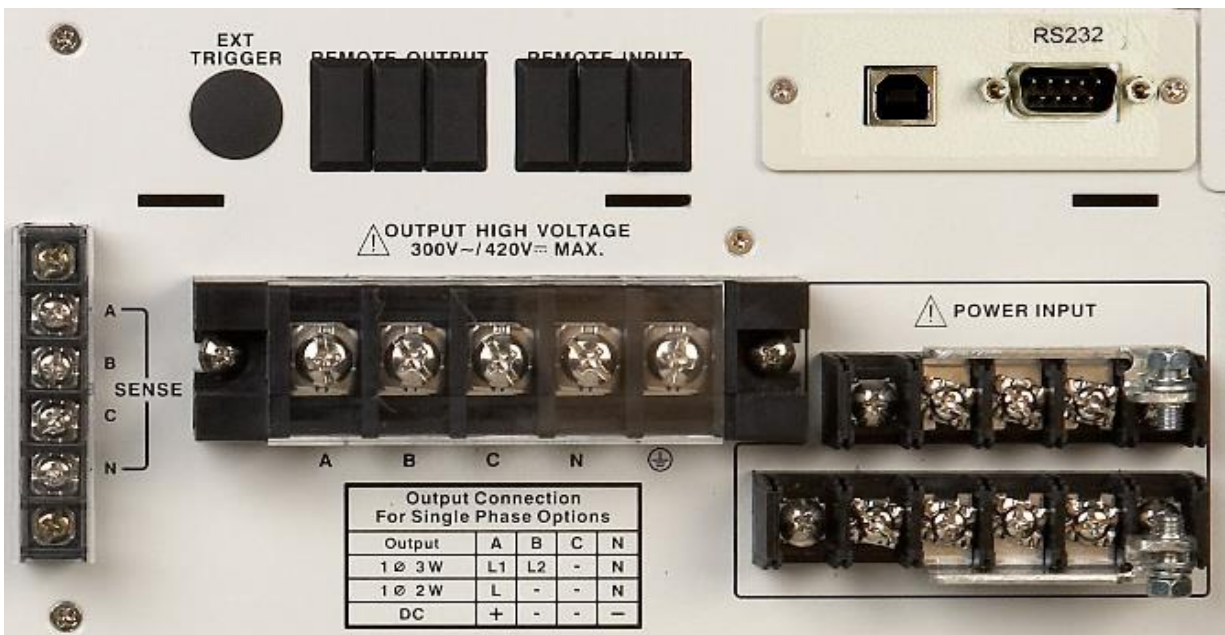
Figure 1: Input/Output Terminal Block and Output Connection Description
