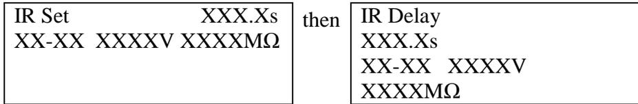
**2.2.** If the DUT has passed the test, the green TEST button will illuminate and a short audible beep will be activated. The display will show:
