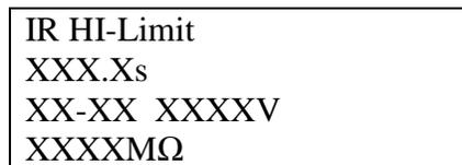
To stop the alarm, please press the RESET button once. The alarm will stop and the display will retain the failure information. The instrument is now ready for the next test. If the RESET button is pressed again, the failure information on the screen will be cleared and the display will indicate the setting data of the previous test.
