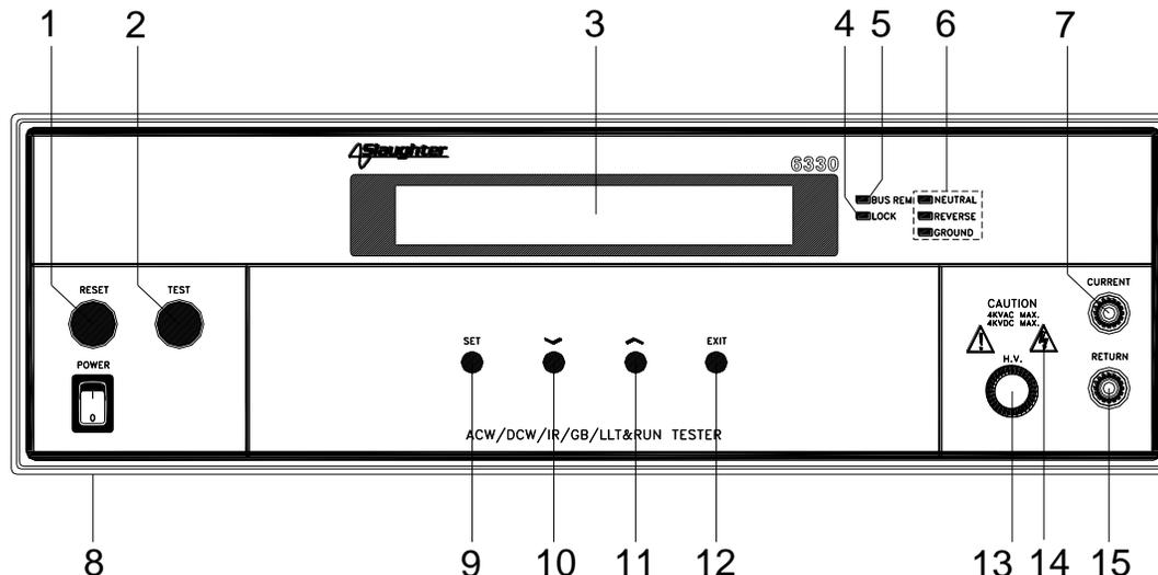
1. **RESET BUTTON:** This is a momentary contact switch used to reset the instrument. If an out-of-range reading is detected during a test, the red failure lamp within the button will light. To reset the system for the next test, press and release this button. This button may also be used to abort a test in progress.
