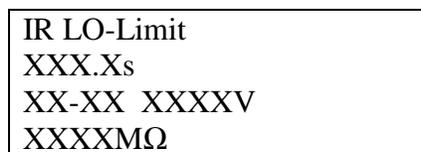
To stop the alarm, please press the RESET button once. The alarm will stop and the display will retain the failure information. The instrument is now ready for the next test. If the RESET button is pressed again, the failure information on the screen will be cleared and the display will indicate the setting data of the test.
