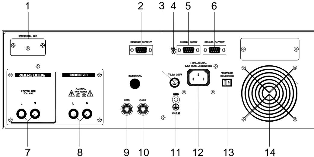
1. **EXTERNAL MD:** Provides an access port for a custom measuring device. The port may be activated during Line Leakage testing from the instrument's menu system. The operator must supply the appropriate measuring device as none is provided.
