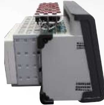
The SENT / PWM factory option is fixed on the back of DAS1600. It provides 20 SENT sensors input and 20 PWM input. P/N: 916009600
