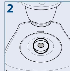
2 Put a specimen on the stage plate
