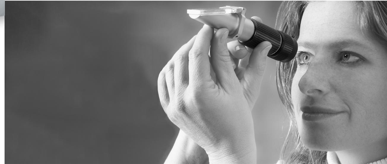
Refractometers are used for the identification of substances and concentration measurements of fluids. Because the refractive index (R.I.) of a solution is proportional to the concentration, it is easy to identify the substance or to measure the purity and concentrations of solutions
