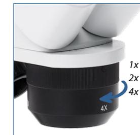
Revolving nosepiece with triple magnification
