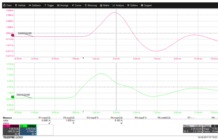
Figure 1: Pulse shape (maximum intensity) ICI 1900 L-EFT
