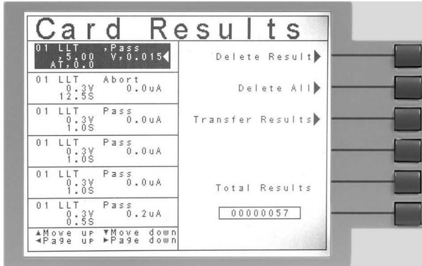
From this menu, the user can view the stored results, delete results, and transfer the results to the external USB Flash memory drive. To navigate through the results use the up, down, left and right softkeys on the 620L front panel. The following message will display if the Delete Result softkey is pressed:
