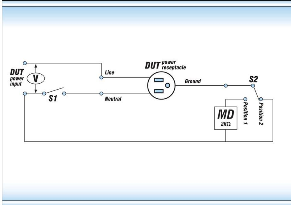
When the Leakage-HI trip limit is set to 0, S2 is placed in position 2 which disables the earth leakage test and connects the neutral of the DUT input to the ground of the DUT.
