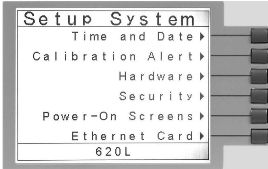
To access the Ethernet Card Menu, press the “Ethernet Card” soft key from the Setup System screen. The Ethernet Card Parameters screen will now be displayed as shown below:
