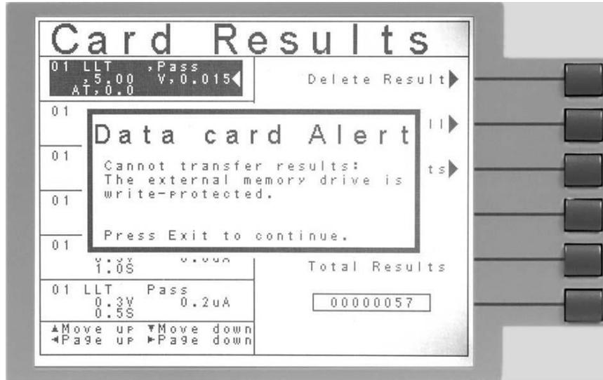
The above message appears when the USB Flash memory drive is write-protected. There are two ways to configure the memory drive as write-protected. One is to set the switch on the side of the memory drive up (towards the drive's connector). The other is to configure it through the drive's properties in Windows.
