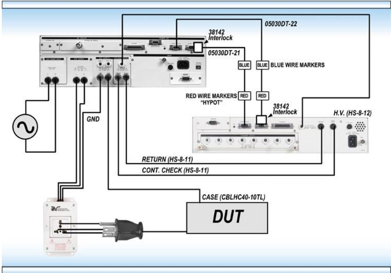
The following figure shows how to connect the 620L to an Associated Research Omnia 8104 tester.
