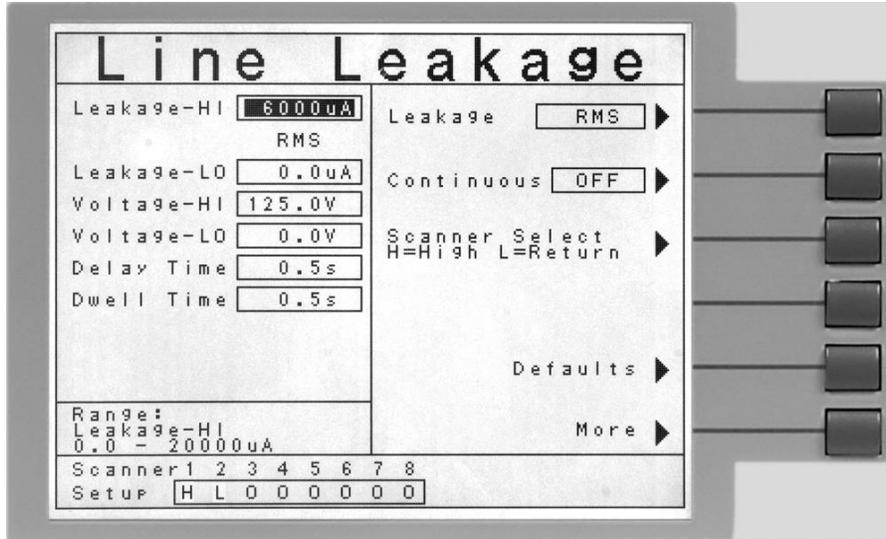
The operator may set the Scanner on a test-by-test basis. For example, for test step 01, the operator may set each of the Scanner channels in a particular configuration. For test step 02, the operator may wish to change the configuration of each Scanner channel.
