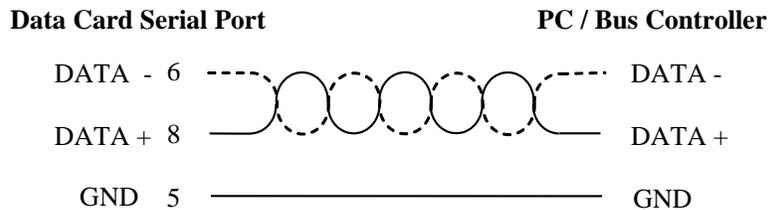
The wire used to connect the DATA signals from the Data Storage Card to the RS-485 network should be twisted pair.
