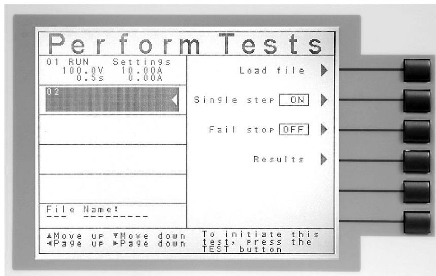
The Perform Tests screen is the main operational screen of instrument. From this screen individual steps are monitored while the test is being performed.
