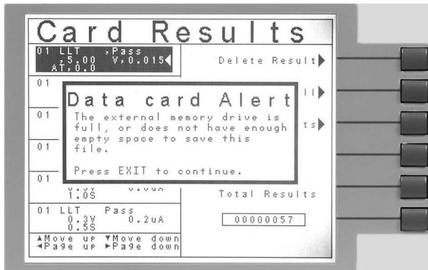
The above message occurs when the user attempts to transfer results from the Data Storage Card onto the USB Flash memory drive, but there is not enough empty space on the drive to save the file. To save the results file, the user needs to create some empty space on the USB Flash memory drive.
