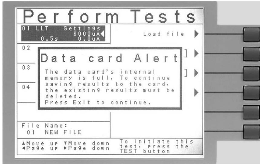
The above message occurs when the total results accumulated on the Data Storage Card exceeds 100,000. The 620L will not allow any more tests to be run unless the user deletes the results currently on the Data Storage Card or changes the Test Result setting in the Data Card Settings menu to NONE. If the Test Result setting is set to NONE, the Data Storage Card will not record test results.
