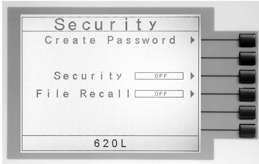
You may create a password from this screen so that all security functions will require a password. From the Security Settings screen, three different parameters may be accessed: Create Password, Security and File Recall.
