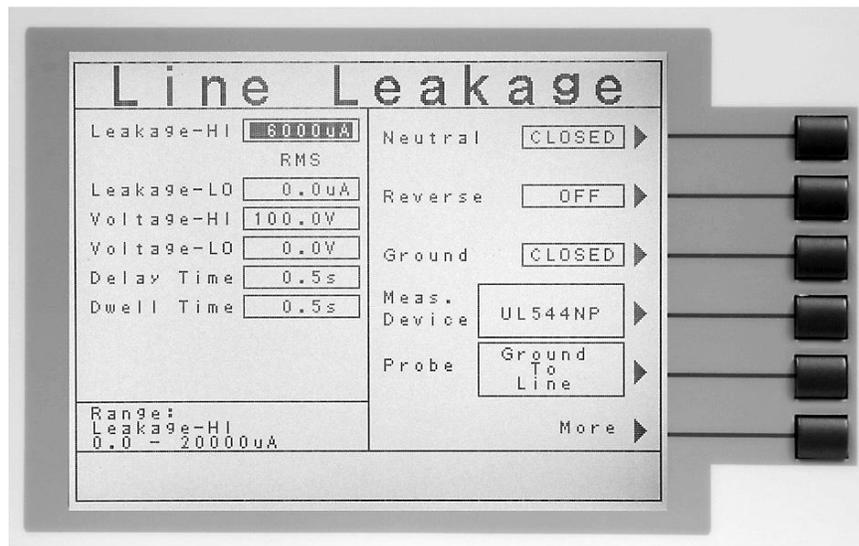
From the Line Leakage Parameter Setting screen, the following parameters may be controlled: Leakage-HI, Leakage-LO, Voltage-HI, Voltage-LO, Delay Time, Dwell Time, Neutral, Reverse, Ground, Measuring Device, Probe, and More. Pressing the “More” soft key will bring up additional parameters: Leakage, Extended Meters, AC/DC, Ranging Mode and Continuous.
