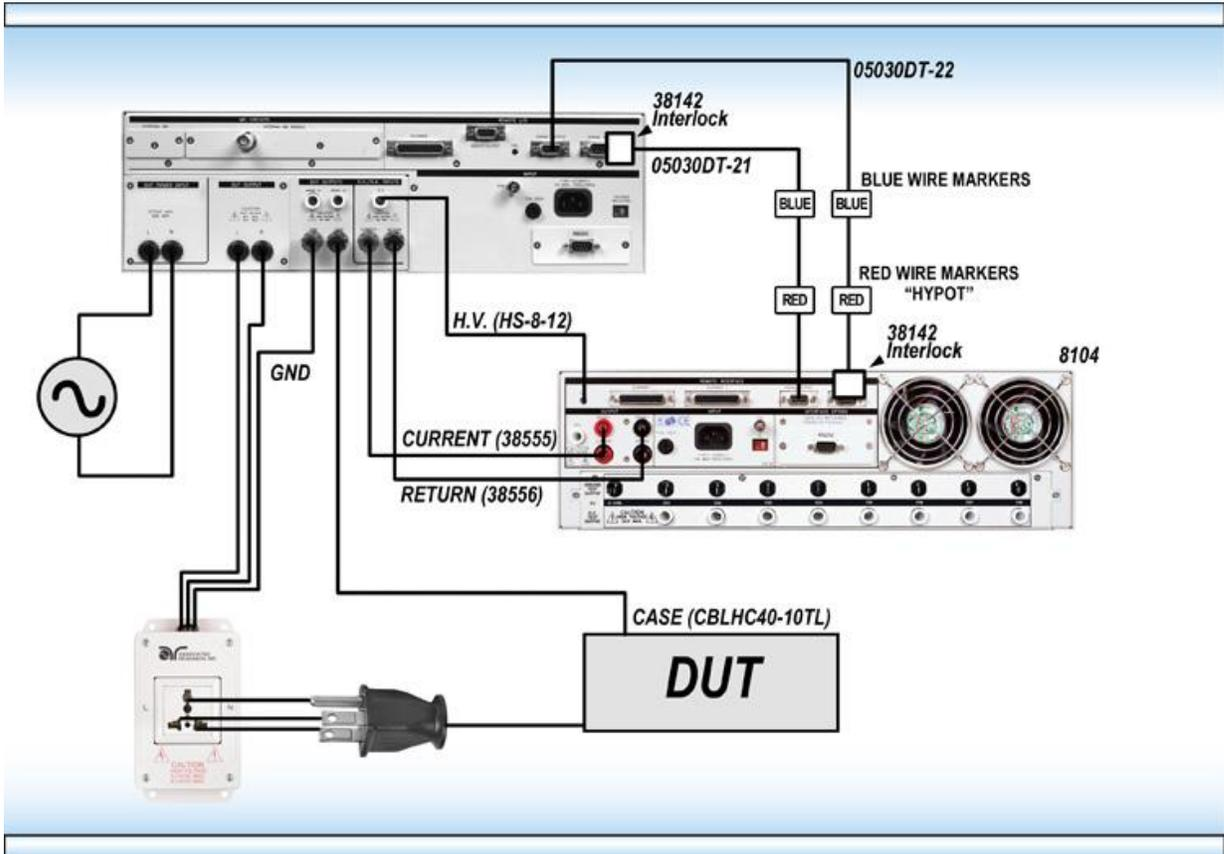
The following figure shows how to connect the 620L to an Associated Research Omnia 8104 tester using special cables to perform hipot test first followed by line leakage test
