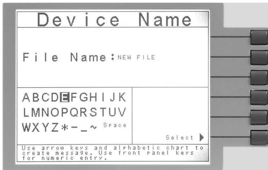
From this screen you may enter a Device Name for the 620L. The Device Name is used to identify the 620L on your server and may be used in place of a dedicated IP Address. Use the arrow keys to highlight a letter and press the “Select” soft key to select the highlighted letter. The Device Name may be a maximum of eight characters and MUST start with a letter. If the Device Name does not start with a letter the following error message will be displayed:
