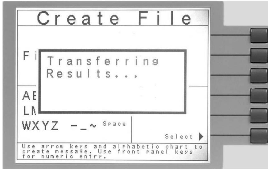
This message will appear on the screen until the Time Remaining reaches 00:00. For each transfer, the Data Storage Card will copy all results in the internal Flash memory regardless if some or all of the results have been transferred before. During each transfer, the Data Storage Card will create a .txt file that will contain the information for all of the results. To view this .txt file, remove the USB Flash memory disk from the Data Storage Card and connect it to a PC with a USB port.
