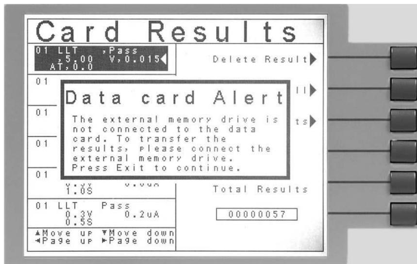
The above message occurs when the user tries to transfer results from the Data Storage Card without the USB Flash memory drive connected. To transfer results, the user needs to have the Flash memory drive connected to the Data Storage Card.
