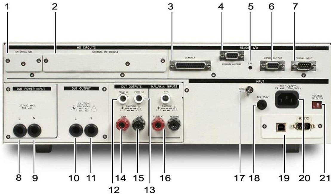
13. **PROBE LO:** Connector used to attach the Probe-LO test lead to the DUT. When used with an appropriate test lead, this terminal connects one side of the MD (measuring device) to the DUT during Applied Part Line Leakage tests. The terminal is always used in conjunction with the Probe-HI terminal.
