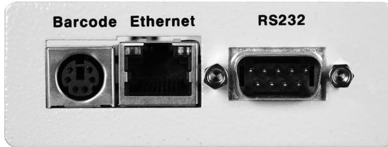
The port labeled “Barcode” is a PS/2-type connector that is used for the connection of a barcode scanner. The Ethernet port is for use with a standard CAT-5 Ethernet cable and may be connected to any compatible PC. The 9-pin D-type subminiature connector labeled “RS232” is for connection of the 620L to an RS-232 communication bus.
