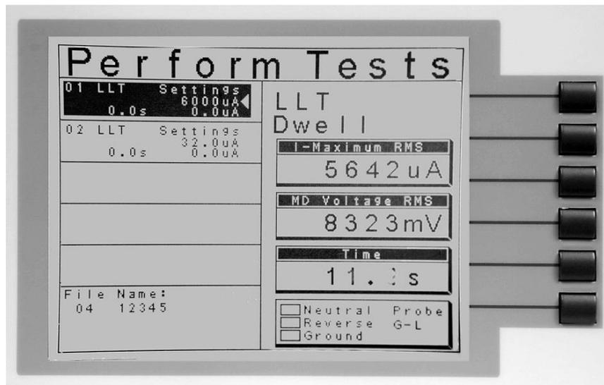
While a Run test is in the dwell phase you may view a series of alternate meters. The alternate meters are: leakage, PF, power and time.
