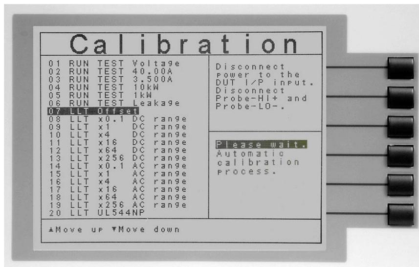
This calibration is automatic and does not require data entry.
