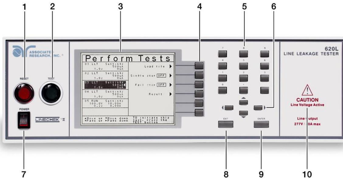
**9. ENTER KEY:** Key used to finalize parameter entries. The ENTER key may also be used to scroll the highlighted area to different parameters in the parameter setting screens.
