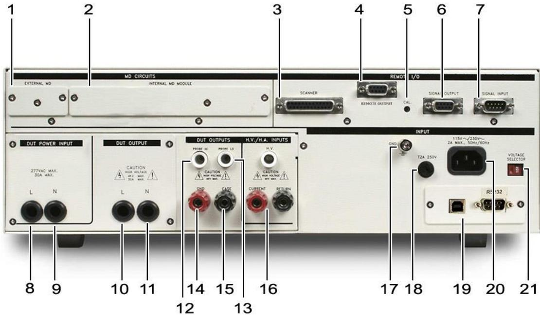
1. **EXTERNAL MEASURING DEVICE:** Contains an external Measuring Device PCB that will enable during a Line Leakage test when “External” is selected from the “Meas. Device” soft key. The external MD allows the operator to configure a custom measuring device using either a simple resistive component or a complex two pole network.
