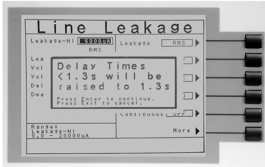
**Ranging Mode:** Unit ranging setting used during the Line Leakage test. Can be set to Auto or Manual.
