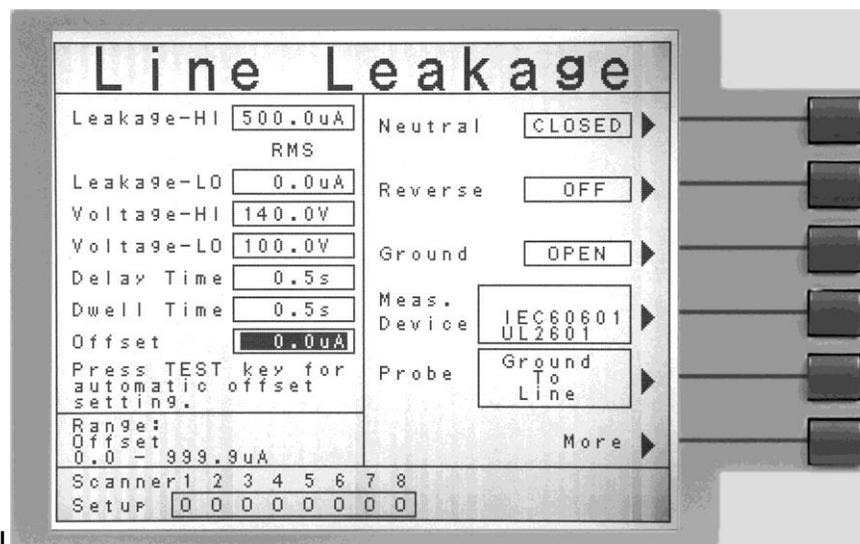
It is recommended that the offset be performed for each line leakage test. This is to account for inherit leakage readings on the system under the various fault conditions. The offset is not universal for the line leakage tests so a reading must be taken on each individual line leakage test.
