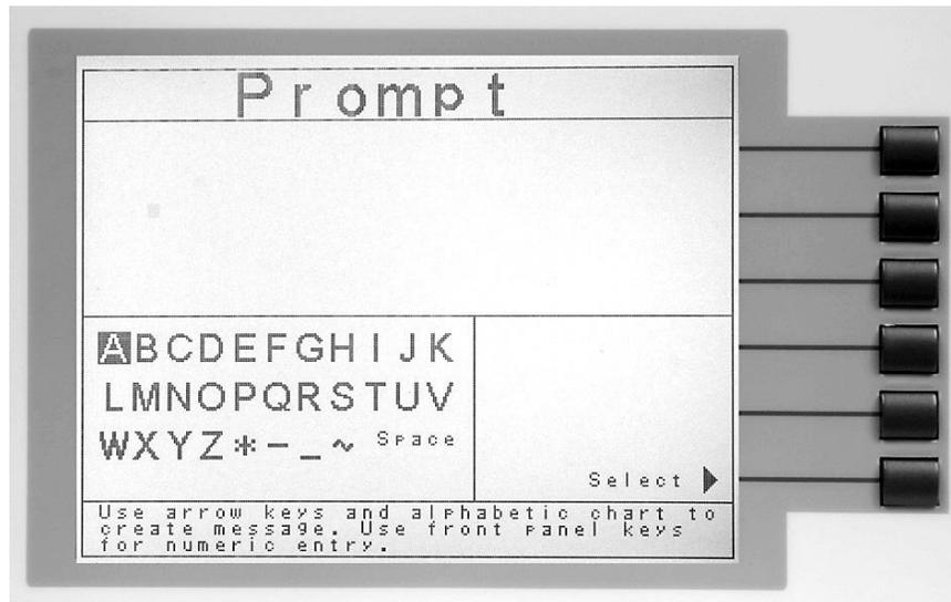
To enter a Prompt use the arrow keys to scroll the highlighted area to the character (or enter a number from the numeric keypad) you wish to use and then press the “Select” soft key. If you make a mistake or want to change the character press the backspace key “←” in the numeric keypad. When you have finished editing the Prompt press the ENTER key. After a Prompt is inserted in a step, a “P” will appear within the step parameters below the step number.
