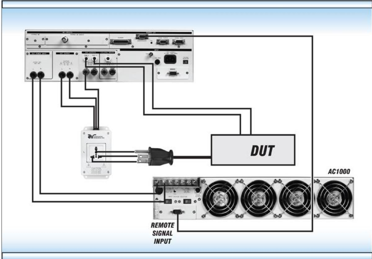
When using this option with an AC 1000, be sure to power up the 620L first and then power up the AC 1000. When powering down the instruments, power down the AC 1000 first and then power down the 620L. The 620L is in an undetermined state without power and may cause inadvertent memory activation of the AC 1000. If you would like to operate the AC 1000 independently of the 620L, either disconnect the interface cable or disable the PLC remote on the AC 1000.
