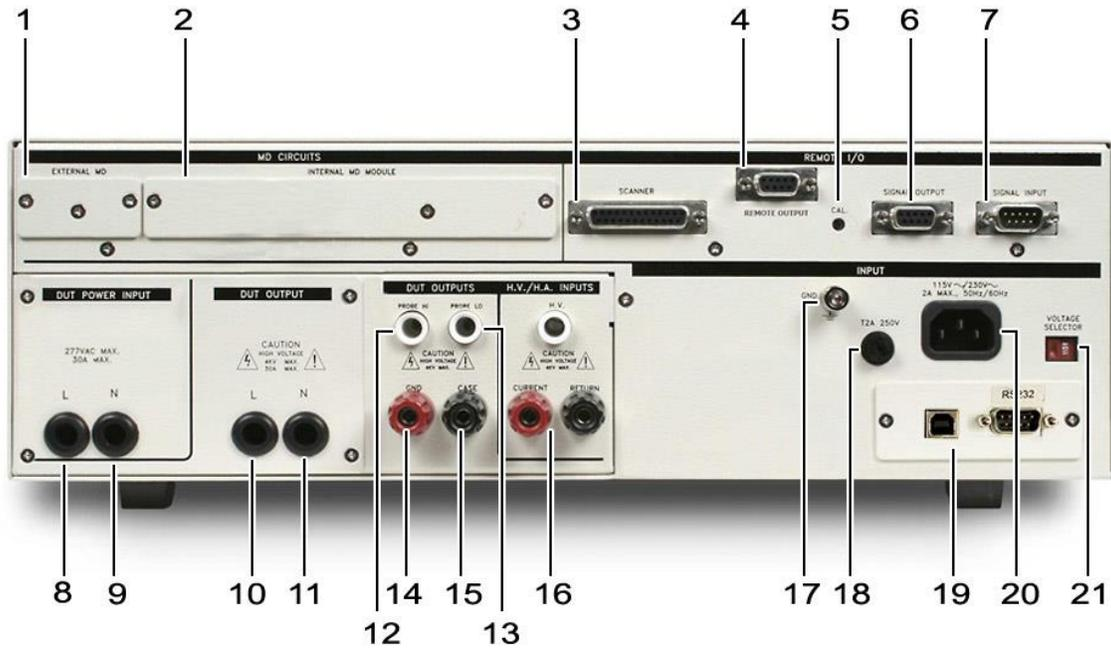
**20. INPUT POWER RECEPTACLE:** Standard IEC 320 connector for connection to a standard NEMA style line power (mains) cord.
