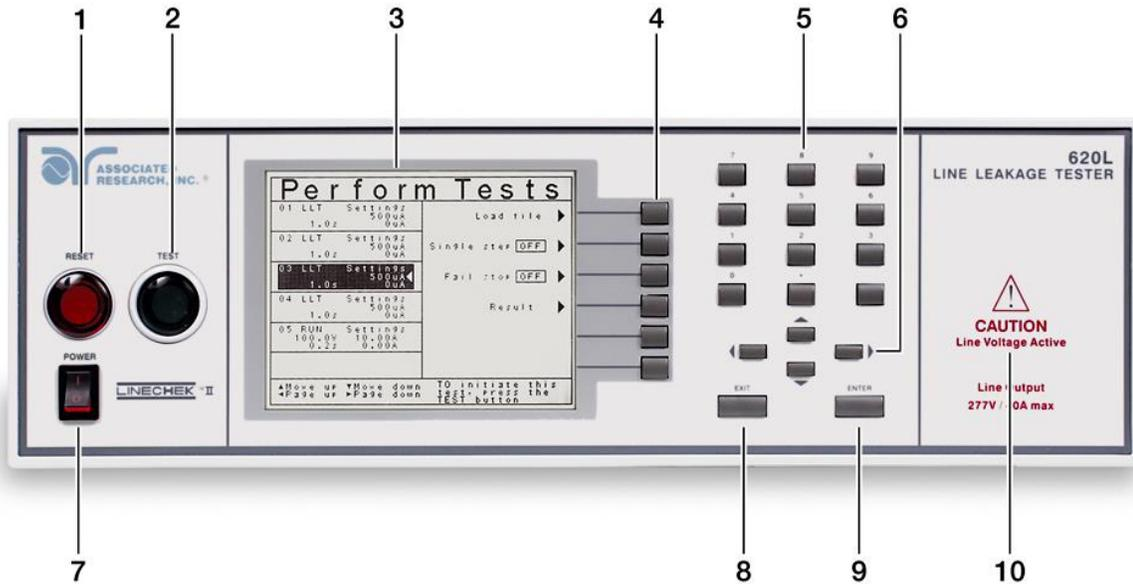
1. **RESET BUTTON:** Resets the instrument. If a failure condition occurs during a test, pressing this button will reset the system, shut off the alarm and clear the failure condition. The Reset button must be pressed before performing another test or changing any of the setup parameters. This button also serves as an abort signal to stop any test in progress.
