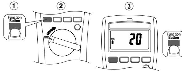
Press the function button and turn the meter on. Then press the function button to select the time. The time can be 5 minutes, 10 minutes, 20 minutes, and disabled (AoFF).
