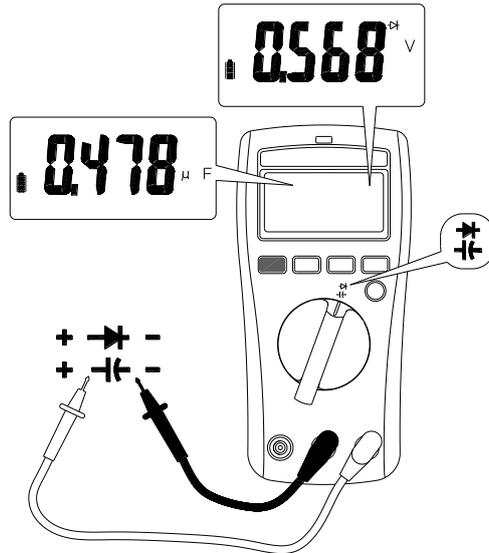
Dial the switch and press the Function button to select the measuring function
