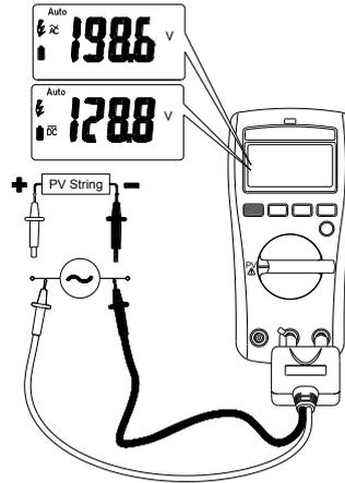
Dial the switch and press the Function button to select the measuring function
