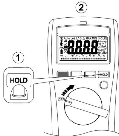
To turn on the meter after keeping HOLD button down.
