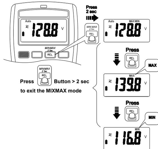
The MAX/MIN mode records the min and max input values. When the input goes below the recorded min value or above the recorded max value, the meter records the new value. Press Hold button to pause the recording.
