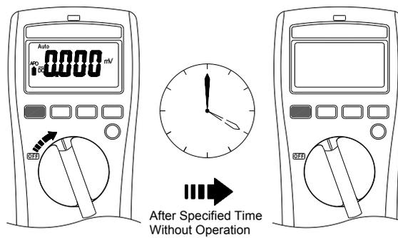
Wake up the meter by dialing the switch or pressing any button.
