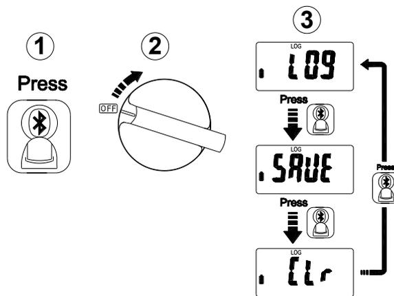
Pressing Bluetooth button while powering-up to select the mode – Data Logger mode, Manual Saving mode and Clear memory.
