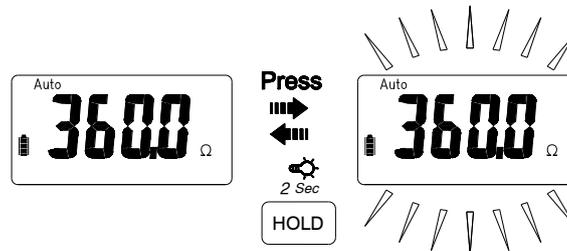
Press the HOLD button over 2 sec to turn on/off Backlight.
