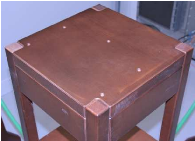
Fig. 13: ES 1530 alignment for calibration loop in horizontal position
