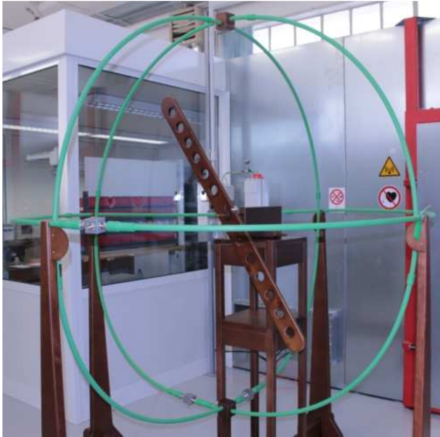
Fig. 19: CS 1530 installation for calibration loop vertical position
