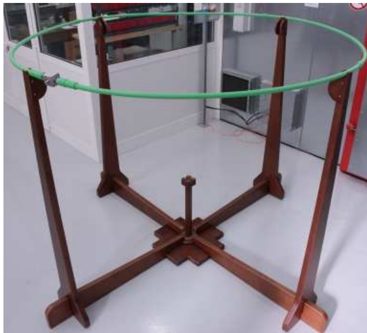
Fig. 6: Horizontal loop installation
