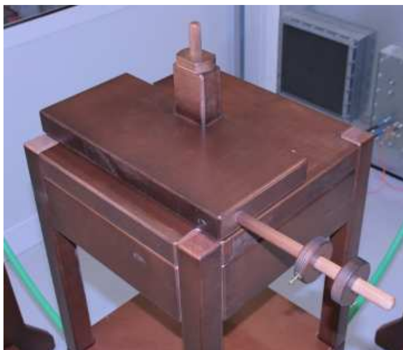
Fig. 14: Support setting for calibration loop in horizontal position
