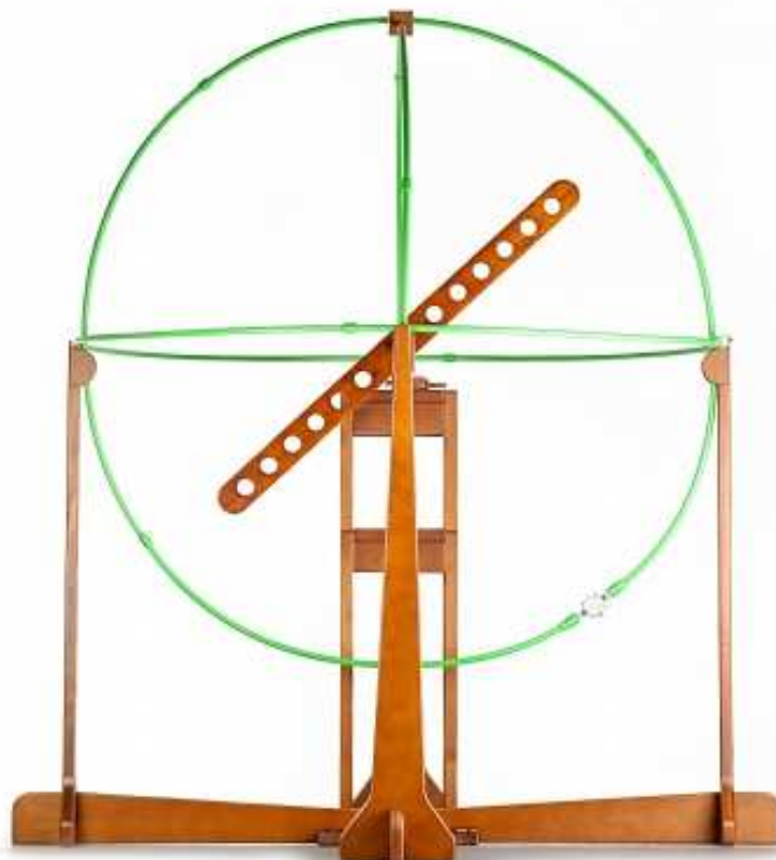
Fig.1: AFJ VVL 1530 Van Veen Loop antenna with AFJ CK 1530 calibration kit inside
