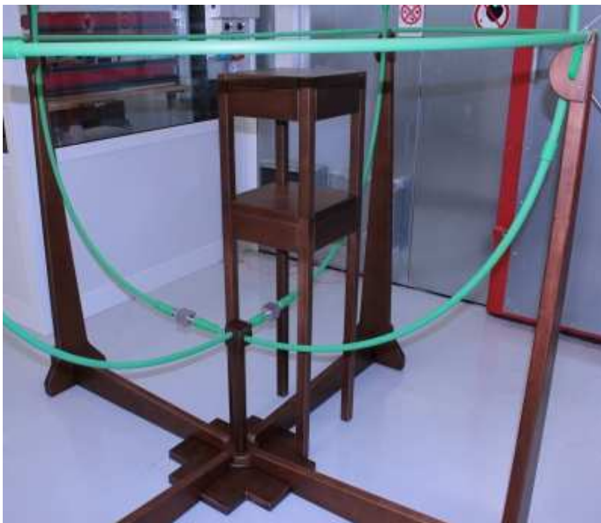
Fig. 16: ES 1530 set within loops for calibration loop in vertical position
