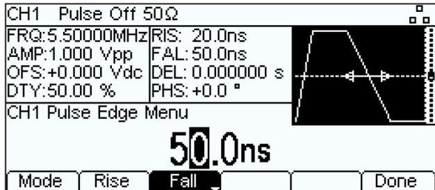
Rise and fall can be set together, or set independently. There are no limitations on rise time imposed by the pulse width.
