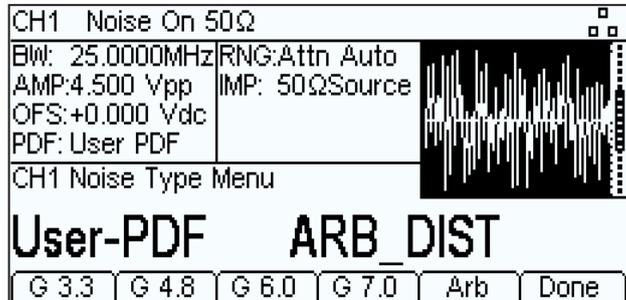
Noise bandwidth can be set anywhere between 0.1Hz and 25MHz (12.5MHz on TGP312x models).
