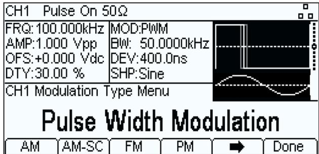
The modulation source can be internal or external. A very wide range of internal modulating waveforms are available.
