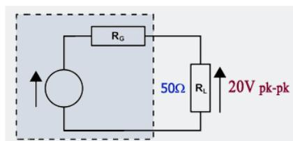
Switchable output impedance allows full load-source matching when levels below 11 volts pk-pk are sufficient.
