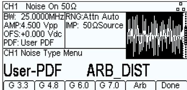
Noise bandwidth can be set anywhere between 0.1Hz and 25MHz (12.5MHz on TGP312x models).
