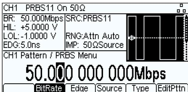
A PRBS is generated by a linear-feedback shift register with taps that generate a feedback signal via an exclusive-OR gate. The number of stages determines the sequence length (2N-1) whilst the clock frequency determines the bit rate.
