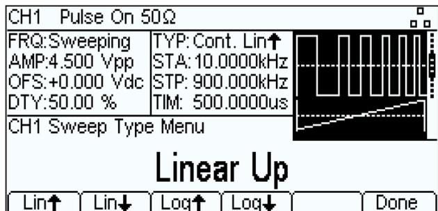
A marker pulse can be generated from the Sync output at any frequency within the sweep span.
