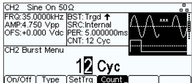
The number of cycles in a burst can be set between 1 and 4,294,967,295 (or infinite). The burst starts and ends at a waveform phase angle settable between -360.0 to +360.0 degrees.
