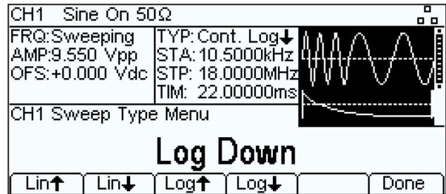
The sweep can be linear or logarithmic, triggered or continuous with a period between 1ms and 500s. The sweep trigger can be manual or internal from the trigger generator or external from the trigger socket or from a remote interface command.
