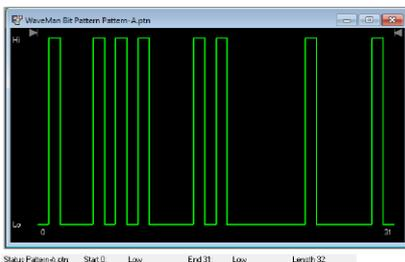
Patterns can be created or edited using the built-in pattern editor, or externally on a PC using the supplied Waveform Manager Plus software.
