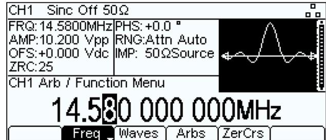
Standard waveforms include Sine, Rectangular, Ramps, Sin(x)/x, Haversine, Logarithmics, Exponentials, Gaussian/Lorentz and Cardiac.
