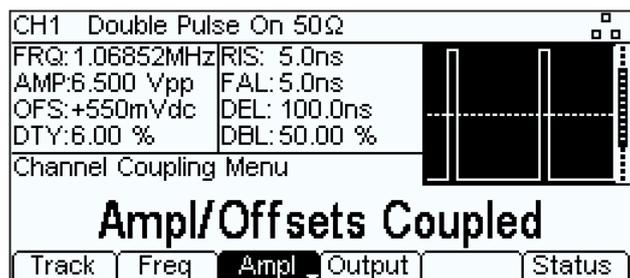
Outputs of the two channels can be coupled such that switching the output on/off on one channel switches the output on/off of both channels.
