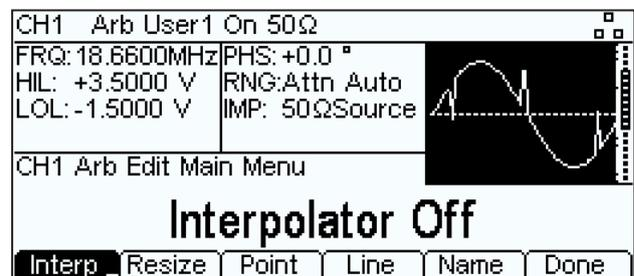
Waveform length is up to 4096 samples. Four waveforms can be stored within the instrument with unlimited numbers available using the Flash drive interface or uploaded from the digital interfaces.
