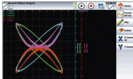
XY mode: your recorder will be a good replacement for your analogue graph plotter. Hardcopy is possible with optional printer.
