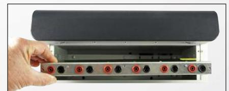
Set up quickly your recorder to match you application: you can use the measurement boards dedicated to your signals (4 different boards can be plugged in).
