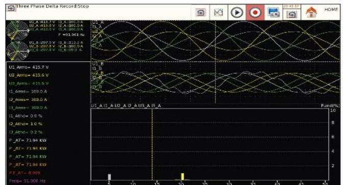
Complete view of recorded parameters. Real time measurement of power, current and voltage. Harmonics are calculated and displayed up to rank 50.
