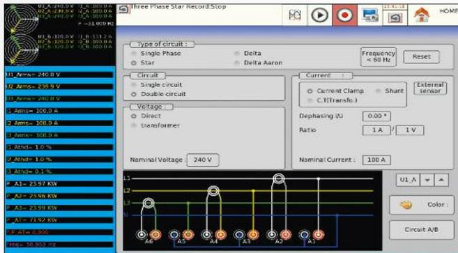
View on a single screen all parameters and measurements for both networks, with two Fresnel diagrams. You can use current clamps selected in the recorder library: all measurements will be calculated and displayed with clamp parameters (transformer ratio).
