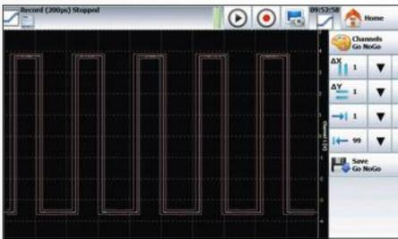
Go-No-Go mode: dedicated for tests on production lines. It is possible to view and record out-of-tolerance signals.
