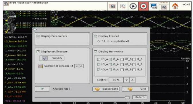
With the setup menu, you can select the parameters you want to measure, display and record.
