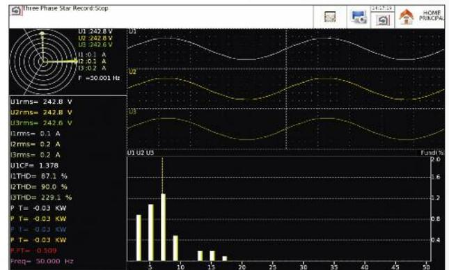
The measurements are operated via current sensors (flexible clamps from 0 to 3000 AAC, or current clamps, or external shunts) and direct voltage inputs (maximum voltage depends on the board used).
