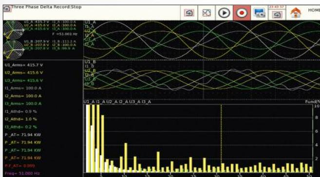
A single screen for all measurements and graphs: voltage, current, power, Fresnel diagrams, harmonics and real time oscilloscope.
