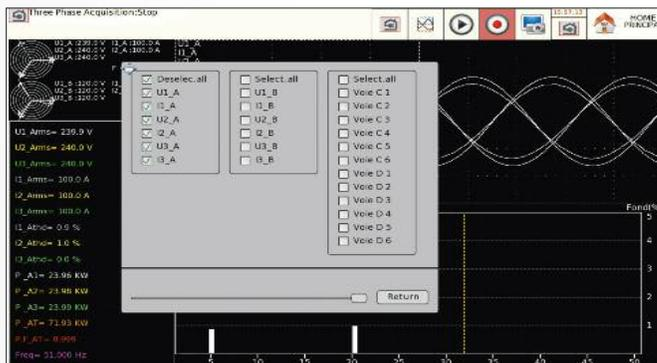
You can select currents and voltages for the oscilloscope mode and the harmonics calculation.
