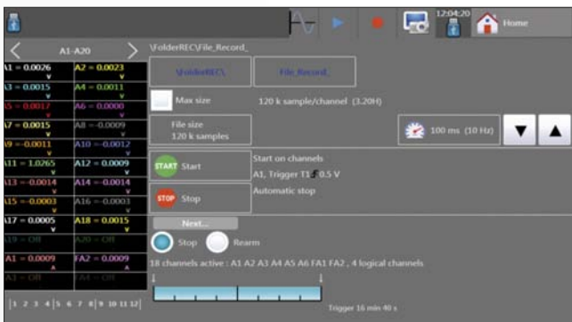
Trigger: multiple choice and combination of threshold, channels and conditions.
