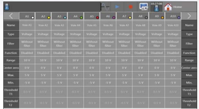
Channels setup: all parameters can be displayed on a single screen.
