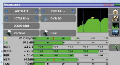
A single screen for all measurements and spectrum.
