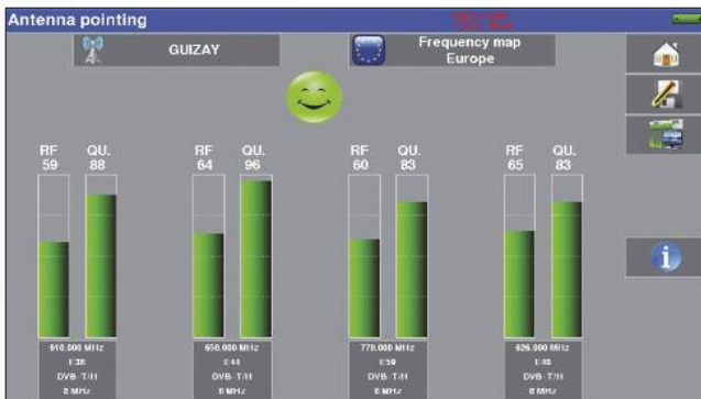
A dedicated function to save time: check sat mode and pointing function for terrestrial.
