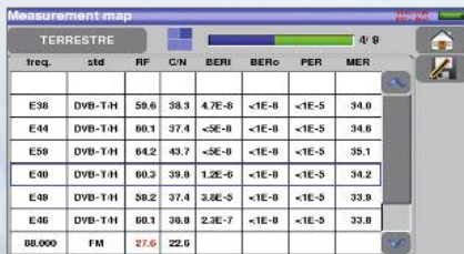
Measurement map for terrestrial, cable and satellite.
