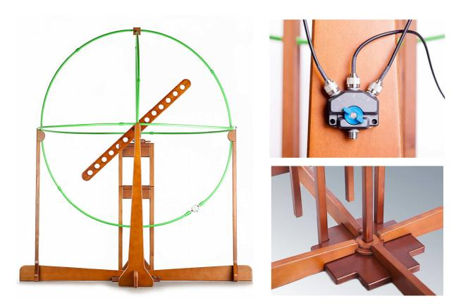
VVL 1530 is a complete 3-axis antenna with a manual switching unit to select each loop in turn. The loops are 2m in diameter with the lowest point 0.5m above ground and are fitted with specially designed current transducers in fully screened housings. Ambient interference is strongly suppressed in open area measurements. VVL 1530 is designed to be collapse down to subunit of convenient size, easy to store. Assembly and disassembly is very fast, no screws necessary.
