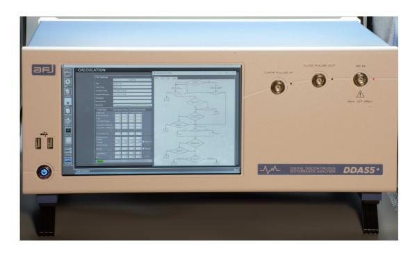
DDA55+ click analyser main characteristic is its ability to sample, in parallel, the Peak and Quasi-peak levels of the four channels, to recognize and count all clicks
