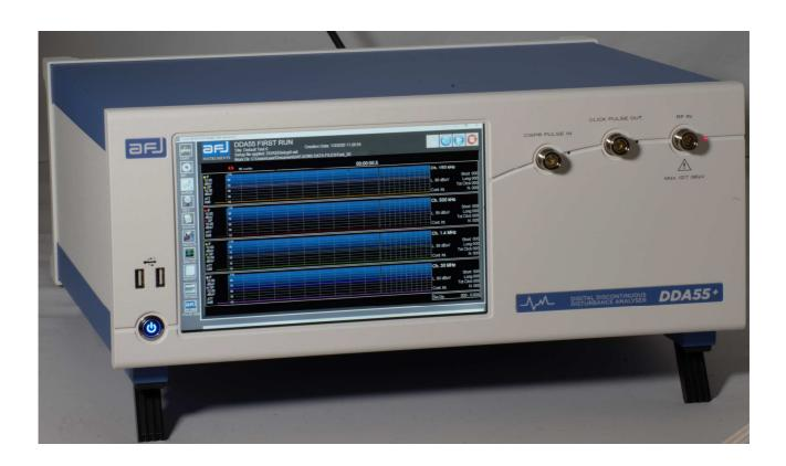
Compact designed and manufactured compliant to CISPR 16 International Standard for measurements of discontinuous disturbances, called "clicks", in accordance with requirements of CISPR 14-1 Standard, advanced software for EMC testing, multi-window real time display, time domain analyse, built-in pulse generator.
