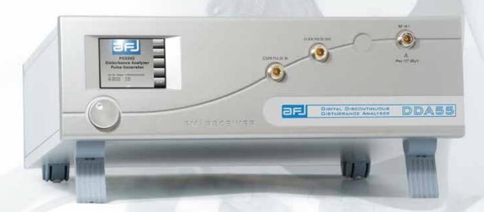
Compact designed and manufactured compliant to CISPR 16 International Standard for measurements of discontinuous disturbances, called "clicks", in accordance with requirements of CISPR 14-1 Standard, advanced software for EMC testing, multi-window real time display, time domain analyse, built-in pulse generator.
