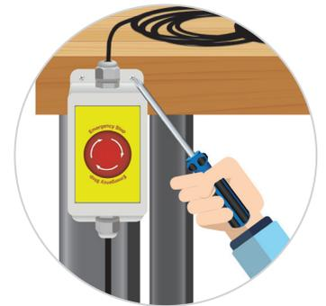
**Step 2** Connect female end of E-Stop to the instrument you wish to control.
