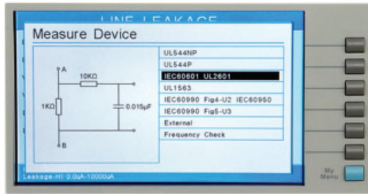
Figure 1: 60601-1 Measuring Device Diagram from OMNIA II
