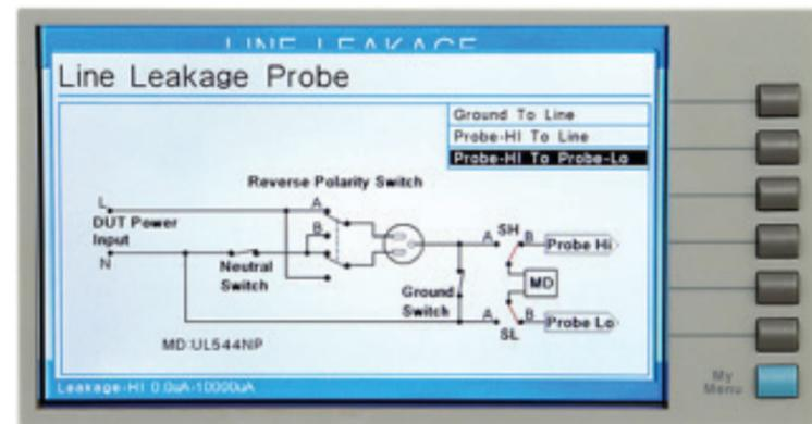
Figure 2: Leakage Current Configuration Diagram from OMNIA II
