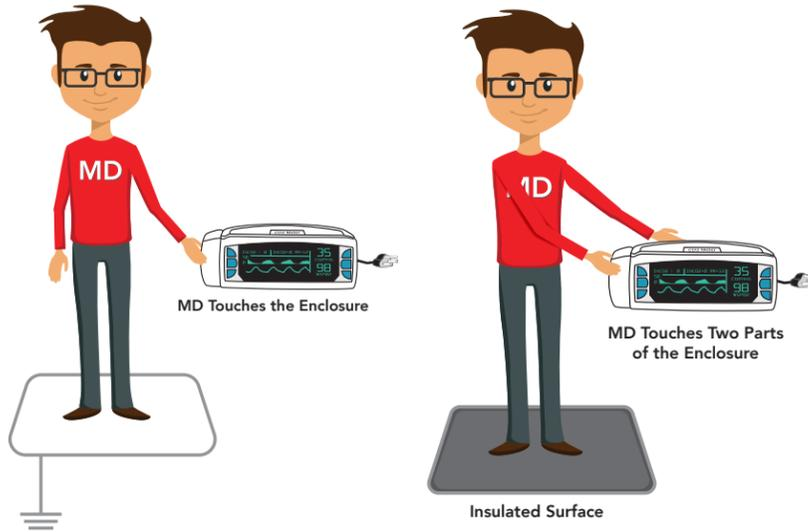
Figure 4 Enclosure Leakage Test
