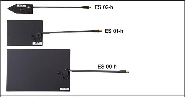
Figure 8 Searching for weak spots with E-field sources
