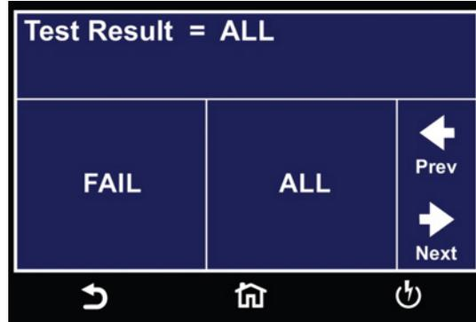
The two options available for Test Result are "All" and "Fail". This option allows you to select which test results will be printed. "All", selects printing all test results and "Fail only", selects printing only failed test results.
