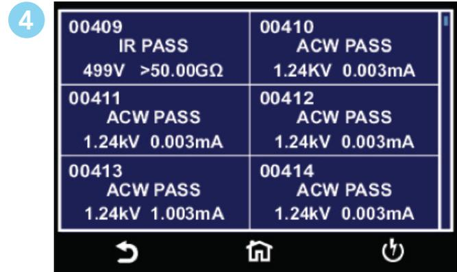
Select Int. Memory to view all the test results stored on the internal memory of the instrument. Scroll down to view all the test results.
