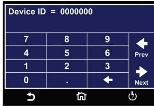
The Device ID number can be entered and saved using the touchscreen keypad.
