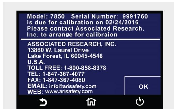
The above Calibration Alert screen will be displayed upon powering up the instrument, on and after the Calibration Alert Date. This screen will display the Calibration Due Date of the instrument.
