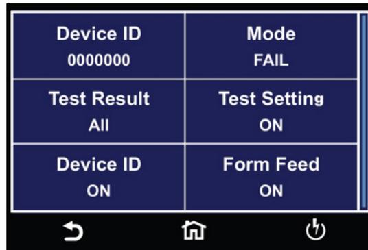
From the Print Format setting screen, six different parameters may be accessed; Device ID number, Mode, Test Result, Test Setting, Device ID, and Form Feed.
