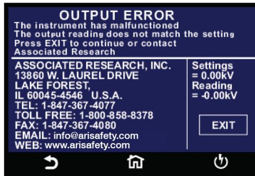
The RESET button is not active in this situation. Only the EXIT button will allow you to return to the Perform Test screen.
