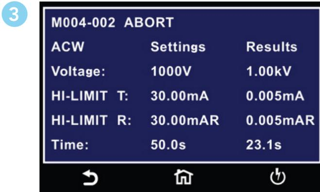
Select Present Test to view test results from the current test sequence that was executed. Select any test step to view more details regarding the test.
