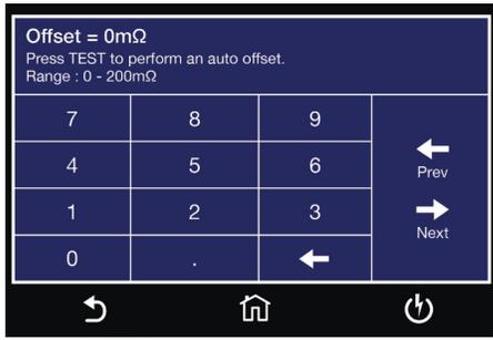
Enter **Offset** value to manually set Offset or Press TEST to perform auto offset.
