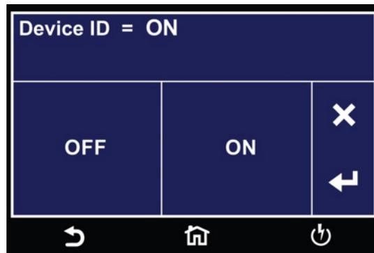
The Device ID number is a counter that increments once every time a test is performed. The number can be set to match the exact serial number or some portion of the actual serial number of the item under test, or just used as an identifier or tracking number. From the Print Format Setting screen select Device ID:
