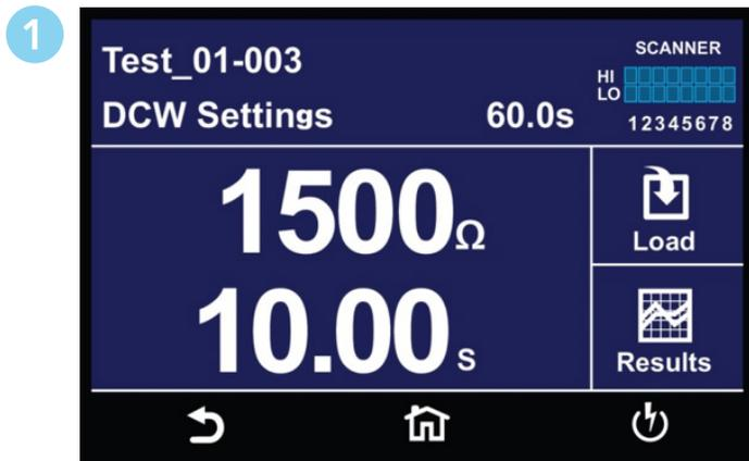
In the image above, the two large meters display the DCW test voltage and the Dwell Time.
