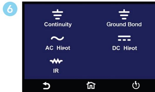
FailCHEK Menu - Check the instrument's failure detectors.
