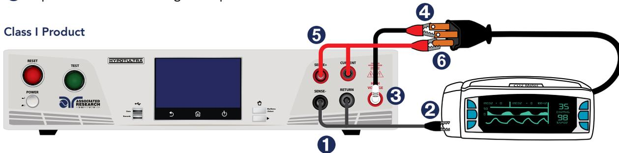
**Did you know?** If necessary, a 10 x 20 cm piece of foil can be attached to the enclosure to simulate a full hand contact to the DUT. This foil acts as the return point. The return and sense (-) terminal are attached to the foil. Always check to make sure you made a good connection between the DUT and the return clip.
