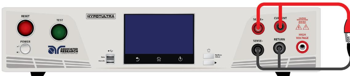
To perform mOhms or Voltage Auto Offset short Red Current/Sense+ Lead with Black Return/Sense- Lead.
