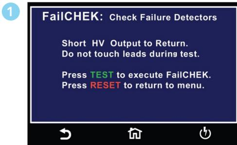
To perform IR Hipot FailCHEK follow on screen instructions and press Green TEST Button or Red RESET to return to previous menu.
