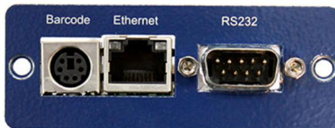
The port labeled "Barcode" is a PS/2-type connector that is used for the connection of a barcode scanner. The Ethernet port is for use with a standard CAT-5 Ethernet cable and may be connected to any compatible PC. The 9-pin D-type subminiature connector labeled "RS232" is for connection of the HypotULTRA to an RS-232 communication bus.
