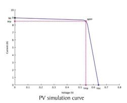
The MR power supply outputs points on the I-V curve in I ms intervals to test the inverter's MPPT efficiency.
