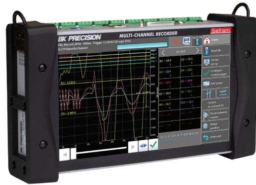
The DAS220-BAT and DAS240-BAT are suited for process control and environmental sensor monitoring.
