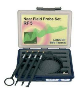
RF5 set Near-Field Probes 30 MHz up to 3 GHz
