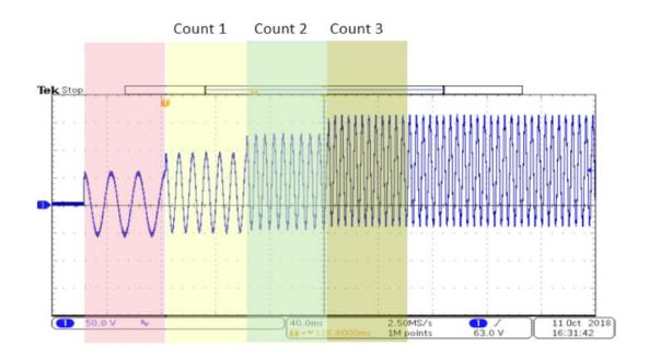
Step Mode allows for the software to program output with multiple counts with each count programmed to setup or step down AC, DC voltage and Frequency. This mode will run test routines according to the parameters currently programmed for each count. The test times are programmed for each count and total test time will Time X Number of Counts. The voltage and frequency output will follow the rate of change listed under dV, dF and dDC parameters.
