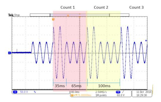
Pulse Mode allows for the software to program output with multiple counts with each count programmed to generate a pulse of change in AC or DC volts. The pulse can be controlled by the Duty Cycle parameter set to a value between 0 and 100 %. This mode will run test routines according to the parameters currently programmed for each count and repeated by the amount of counts the test Period is programmed for. Each count and total test time will be Period X Number of Counts.
