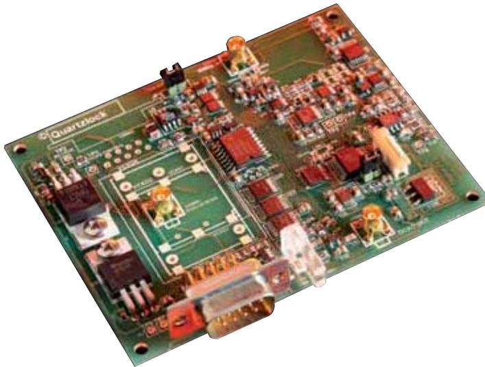
The A6-CPS digital phase locked loop (PLL) provides an low noise, very high short term stability filtered output which can be customised to a specific application. The A6-CPS digital PLL may be fitted into the Quartzlock A6 frequency convertor with BVA OCXO, rubidium, GPS or other options.
