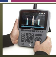
The **HSA-Q1** is a fully integrated portable RF Spectrum Analyser for professional countermeasures use (TSCM). It has been designed with the highest possible technical specification to ensure maximum detection capability and has a range of invaluable features to aid countermeasures RF detection or 'Sweeps'. Easy to use despite capability with added advantage of autonomous portable use.
