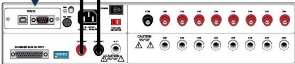
OMNIA 8200 Series and SC6540 Main – Line Leakage Testing 2 SCANNER BUS CABLE (38592)
