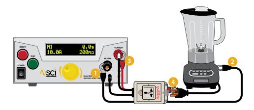
Connect the Interlock Disable Key (P/N 38075) to the Signal Input connector on the rear panel of the tester. If you're not utilizing a DUT enclosure (P/N 39067) or other safety device, <u>the Interlock Disable Key is required in order to run a test.</u>
