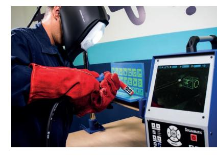
Soldamatic is the first AR welding simulator worldwide, which together with the Augmented Learning Management System (ALMS) based on the concept of Augmented Training, allows training future qualified welders in a more sustainable and efficient way, saving time and reducing costs.
