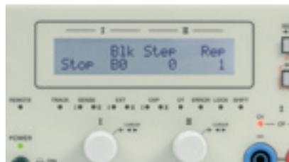
Display of sequence with output of current block, currently executed step, and number of busts of the current block.
