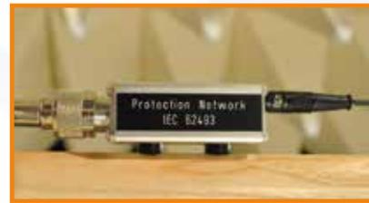
The EMI receiver measures a voltage across 50Ω. It must be connected to the N connector of the protection network. To determine the compliance of a luminary to the standard the measured voltage must be converted into induced internal electric field.
