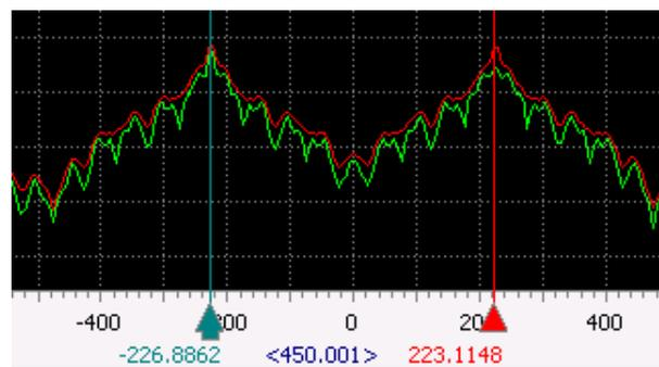
Figure 126.: Spectrum with Peak Hold Curve
