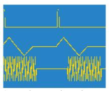
Output signals in trigger and gate modes
