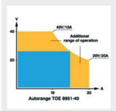
Example: TOE 8951-40 (40 V / 20 A) compared to a standard power supply with 400 W output power.
