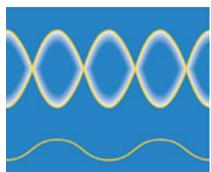
Amplitude modulation with suppressed carrier
