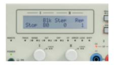
Display of sequence with output of current block, currently executed step, and number of busts of the current block.
