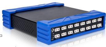
The EX1401 delivers accurate and highly repeatable thermocouple (±0.20°C) and voltage measurements by implementing fully integrated signal conditioning, 24-bit ADC's, and independent Cold Junction Compensation (CJC) on a per-channel basis.
