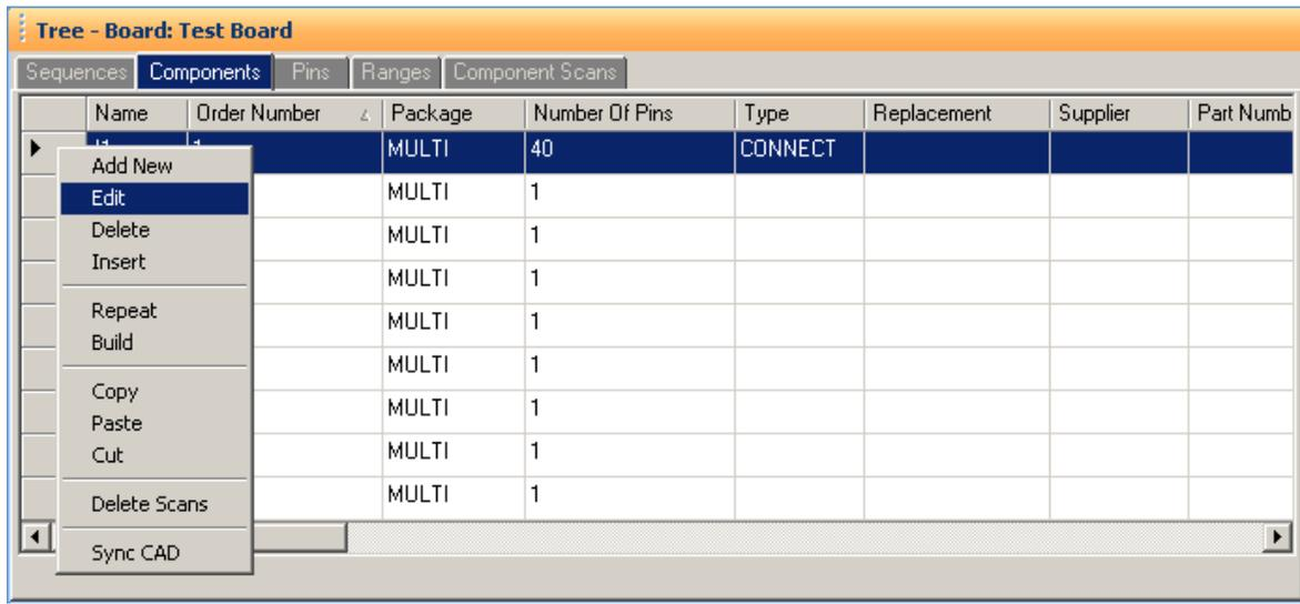
Right clicking on the Row header bar of the Tree pane displays an additional menu for performing specific tasks such as **Add New**, **Insert**, **Delete**, **Repeat**, **Build** (repeat but with name incremented by 1), **Copy**, **Paste** and **Cut**. Right clicking works at all levels of the Tree pane including Sequence, Component (shown above), Pins, Ranges and Scans.
