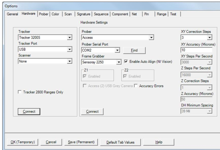
Select **Options** from the **Tools** menu. Select the **Hardware** tab and set the type of Tracker hardware as Tracker 3200S and the Tracker Port as USB. Disregard the Prober settings on the right side of the window.
