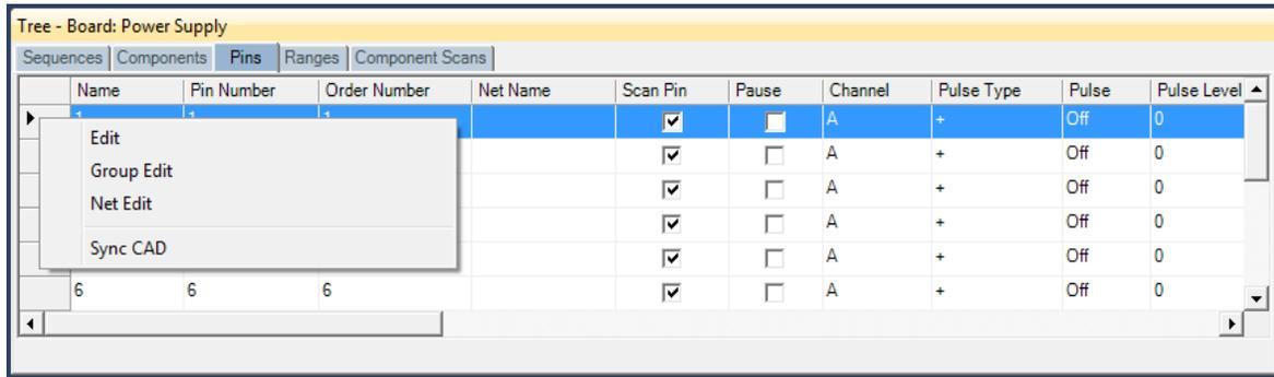
Right clicking on the Row header bar of the Tree/Pins pane allows for editing of the pin information. Select **Edit** to open the Edit window for the selected pin.
