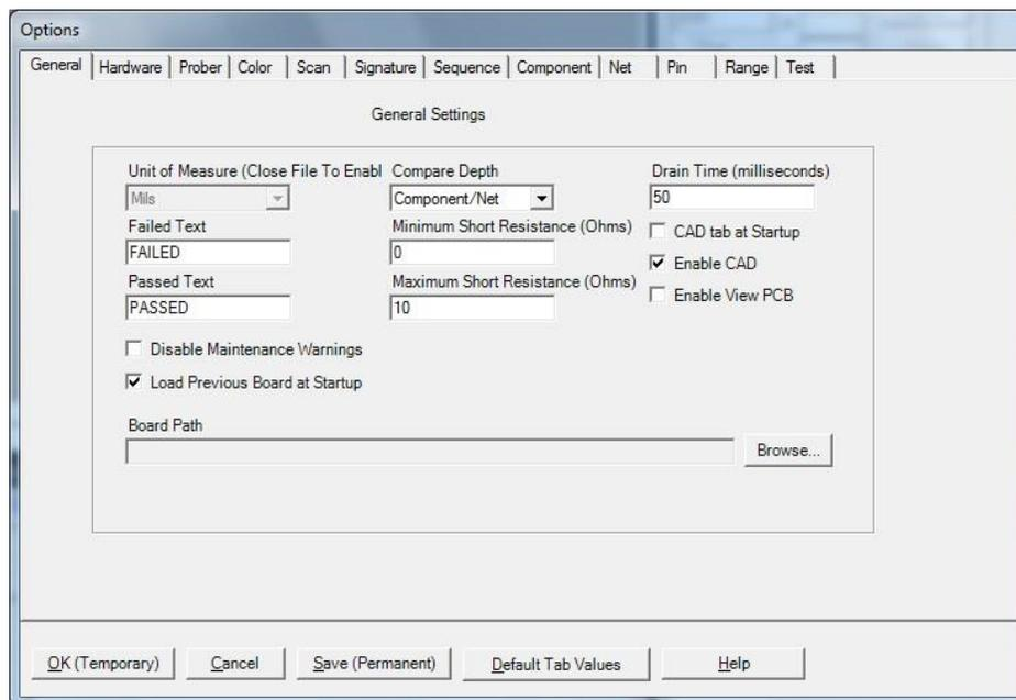
When first starting Huntron Workstation, select **Options** from the **Tools** menu. The Options window is used to setup default settings used when working in Huntron Workstation.
