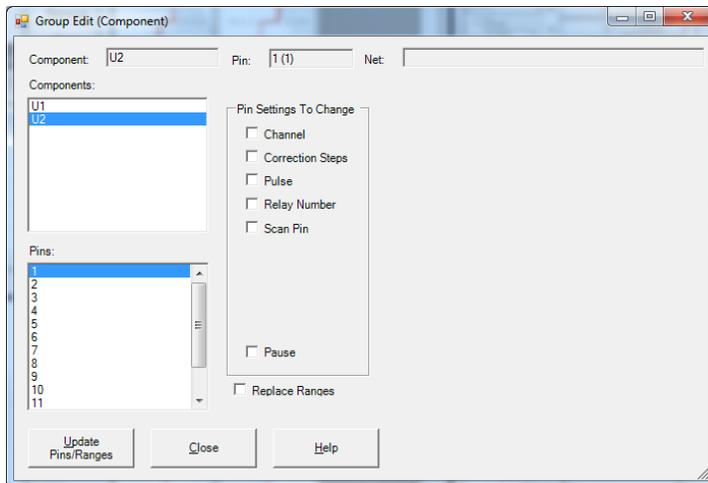
Change the desired settings for the current Pin **first** then select Group Edit from the right-click menu (see above). Components with the same number of pins will be listed. Select the components and pins you want to be changed. Select the Pin Settings check box(s) for the setting(s) you want changed. Check the Ranges box to match the ranges (this will cause signatures to be deleted). Click the **Update Pins/Ranges** button to make the changes.
