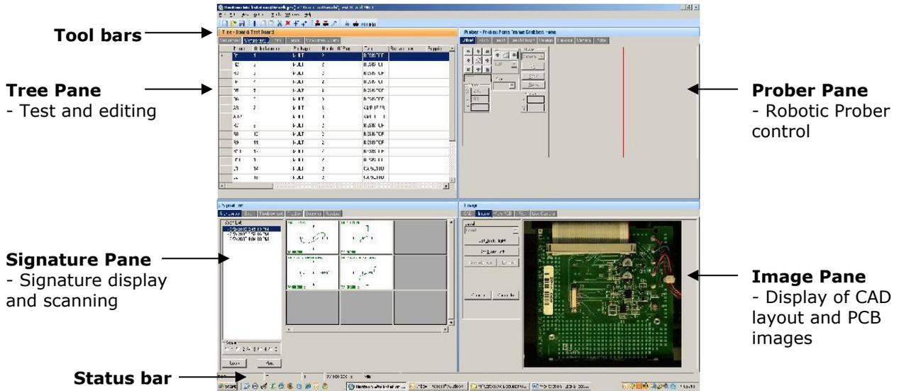
The Main Window for Huntron Workstation 4 features a multi-pane layout so many aspects of the test creation and execution can be displayed at the same time. The Panes are interactive to a certain degree in that changes in one Pane will affect other Panes. The Panes can be resized, floated independently or "tabbed" to the sides of the window. The Status Bar displays information about items currently selected and status information while processes are running.
