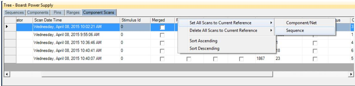
Right clicking on the Column bar of the Component Scans pane displays an additional menu for performing specific tasks such as sorting or globally setting parameters. The menu will vary depending on the column selected. In the image above, the Reference column header was right-clicked.
