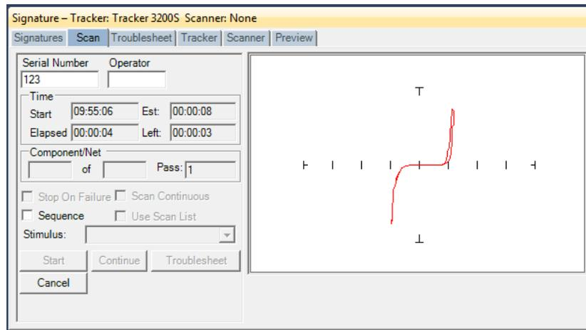
You will be prompted to connect to the component. Tracker with Scanner users should connect to the selected component at this time. Click **OK** to initiate the Scan.
