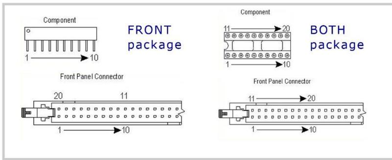
Tracker 3200S scan packages are BOTH, DIP, FRONT, MULTI (used with Probers only), PROBE, SIP, DIP2X, and SIP2X
