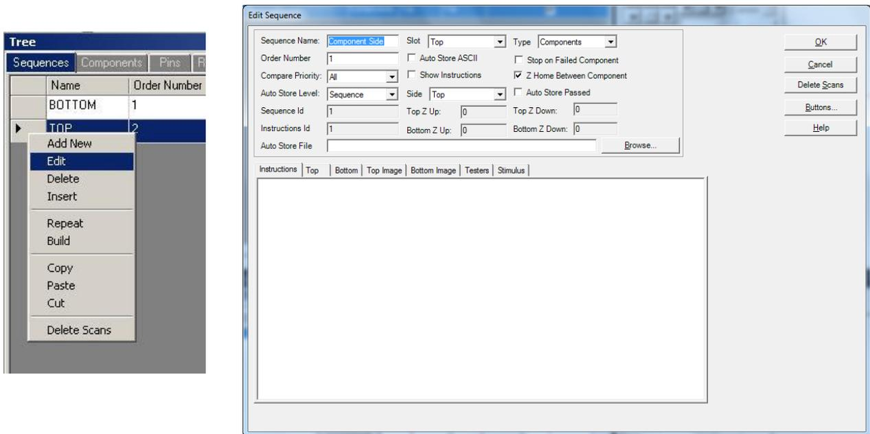
Select the **Buttons...** button located on the right side of the Sequence Edit window to open the Buttons Setup window.
