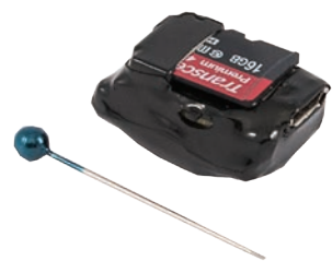
GEM ATOM PLUG AND PLAY: Size: 1 x 2 x 1,4 cm including a 80mAh re-chargeable battery.
