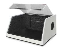
Outside dimensions (W x D x H): 24" x 19" x 11.5" (610  $\times$  483  $\times$  293 mm) Inside dimensions (W x D x H):20" x 16" x 10" (508  $\times$  407 x 254 mm) 3/4" Walls, 3/4" Flame Retardant Foam, 1/4" Plexiglass cover
